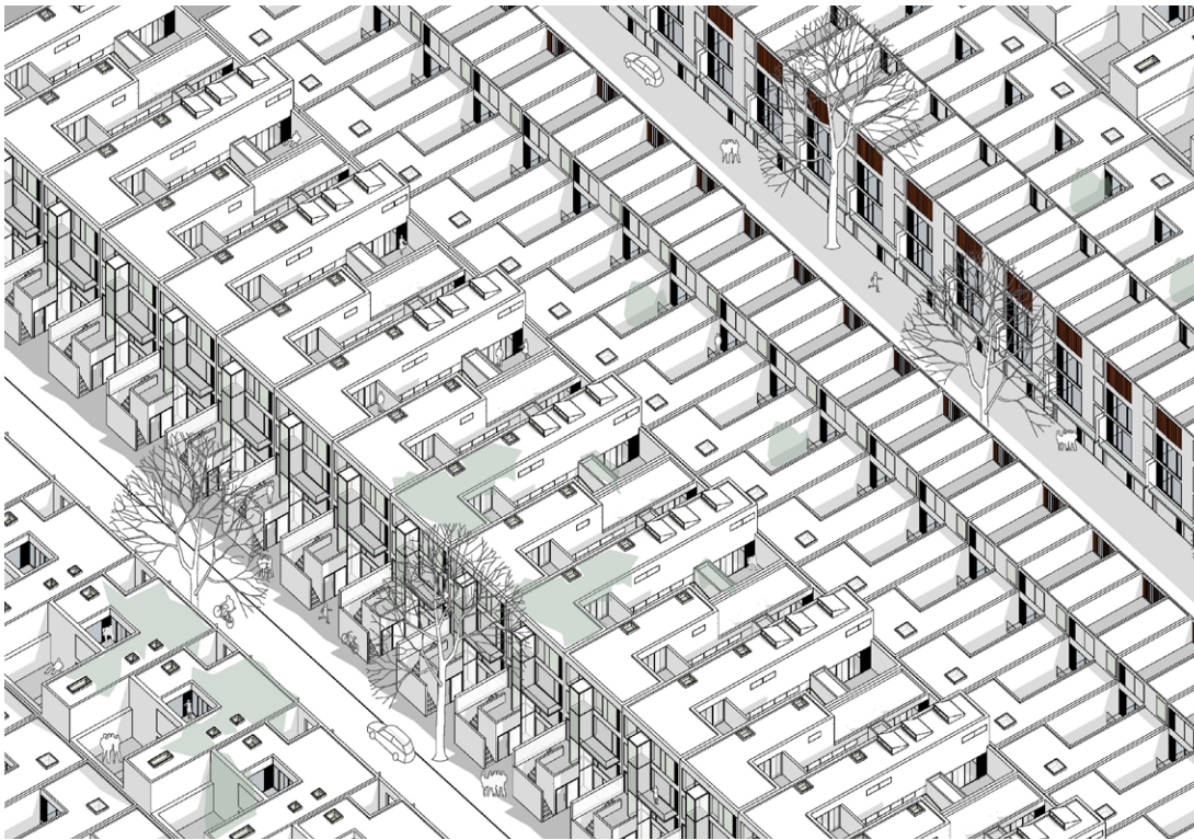
Fig. 2: Isometric axonometry of a conceivable quarter by adding compact courtyard houses on plots of different sizes and proportions. The variants, which can be combined without problems and in manifold ways on three closed sides / outer walls to form an urban complex with corresponding infrastructure and offerings, are part of a common strategy and typology.
